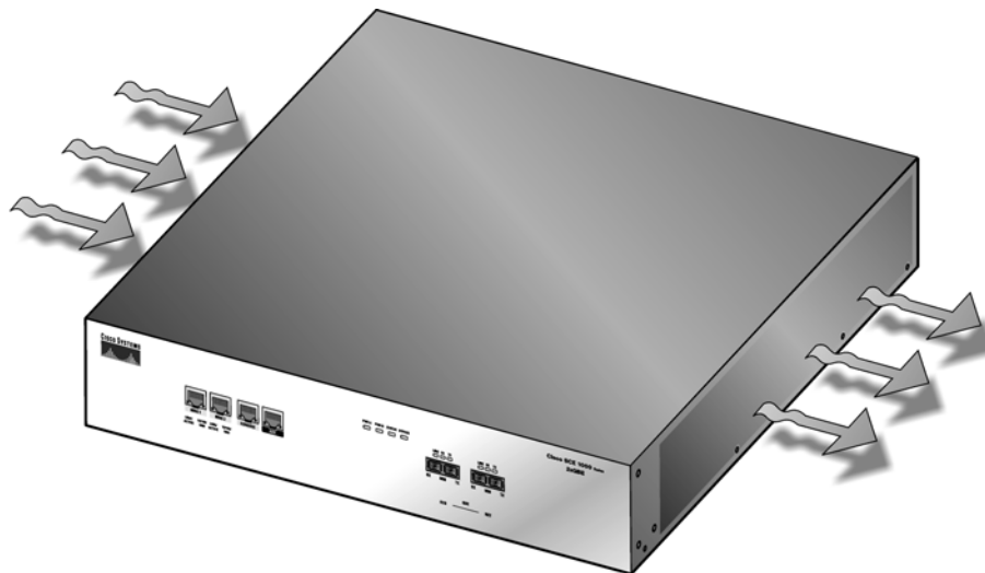
Figure 4-2: Airflow Through the SCE 1000
