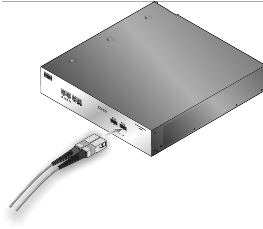
Figure 6-3: Cabling the GBE Interface
