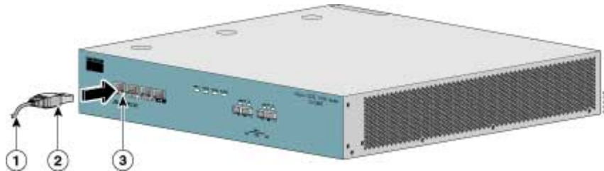
Figure 5-2: Cabling the Management Port
