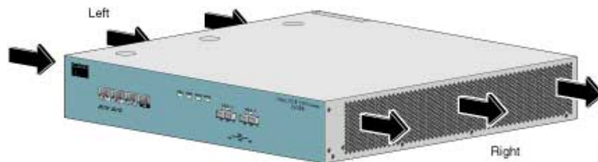
Figure 4-2: Airflow Through the SCE Platform
