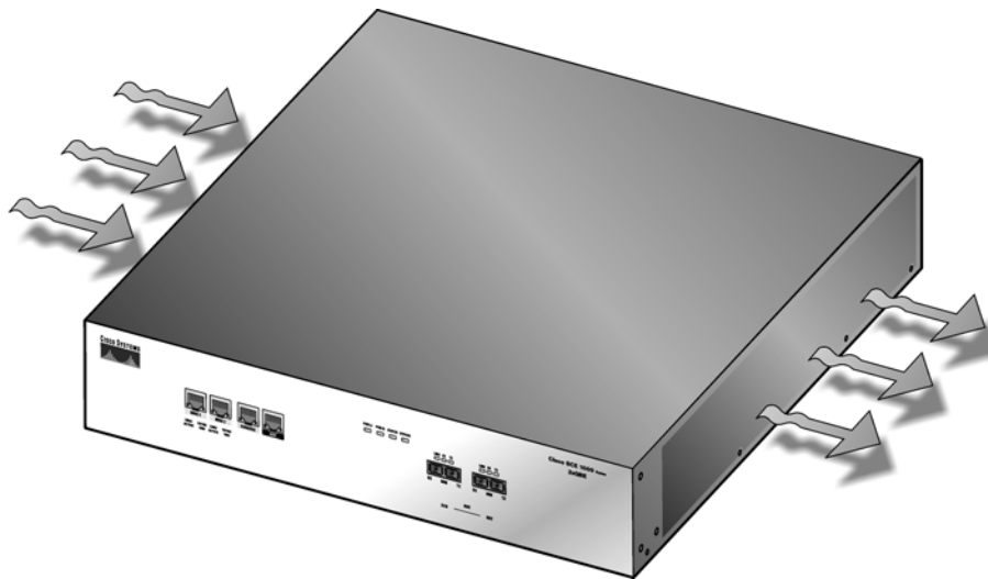
Figure 4-2: Airflow Through the SCE 1000
