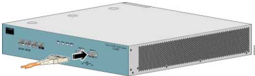
Figure 6-3: Cabling the <ETH> Interface
