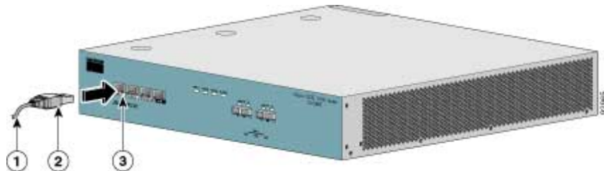
Figure 5-2: Cabling the Management Port
