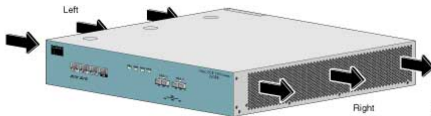
Figure 4-2: Airflow Through the SCE 1000
