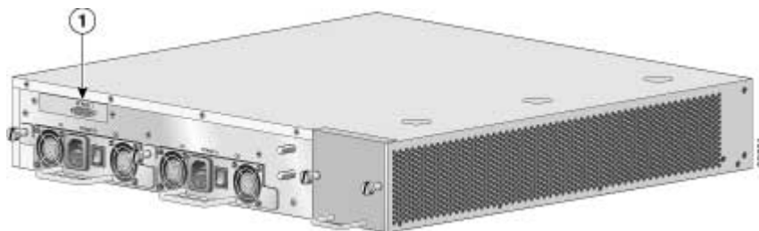
Figure A-4: Bypass Connector on the Rear of the SCE 1000
