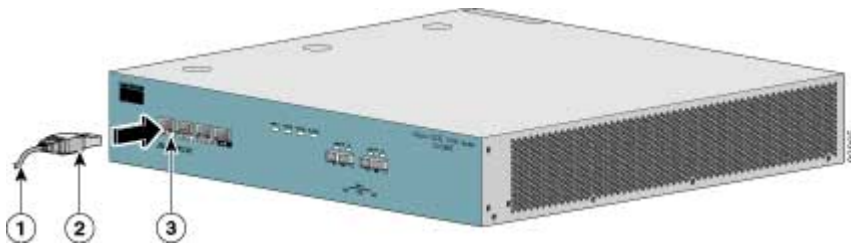
Figure 12: Connecting to the Local Console
