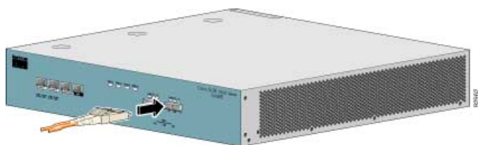
Figure 16: Cabling the GBE Interface
