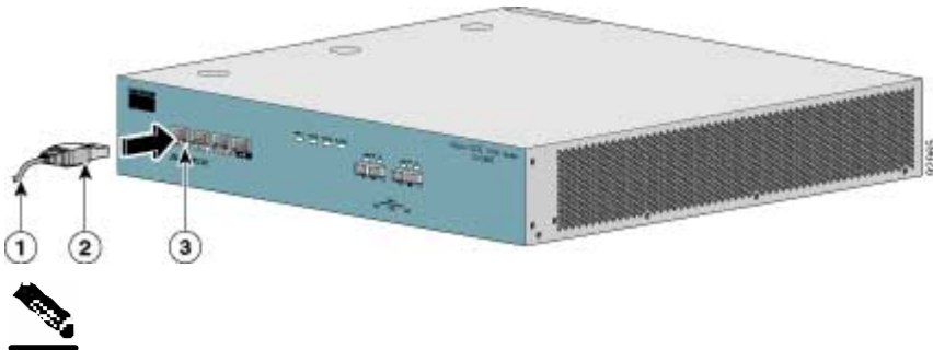
Figure 13: Cabling the Management Port
