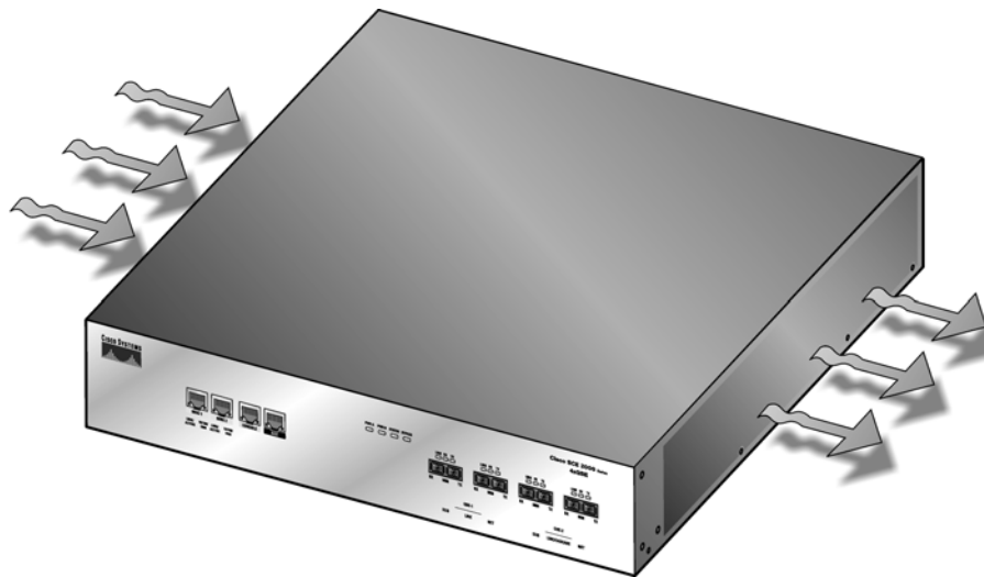
Figure 4-2: Airflow Through the SCE 2000
