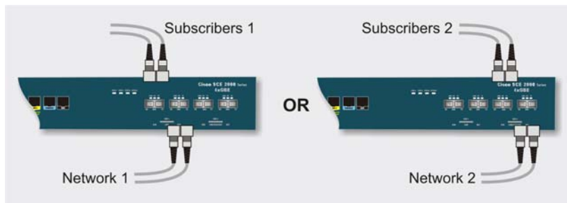
Figure 6-1: Cabling Diagram for Single Link Inline Topology
