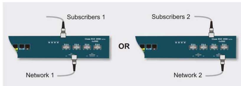
Figure 6-2: Cabling Diagram for Single SCE 2000 Single Link Receive-only Topology
