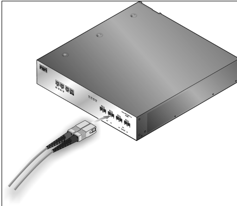
Figure 6-6: Cabling the GBE Interface
