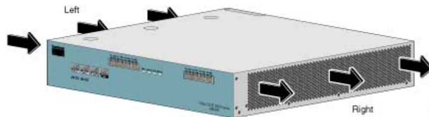
Figure 4-2: Airflow Through the SCE 2000
