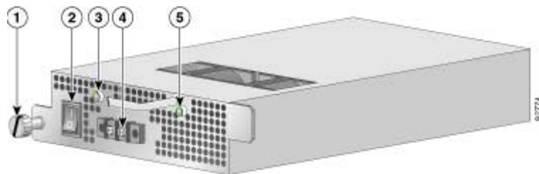
Figure 4-13: DC Power Module
