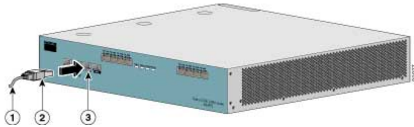
Figure 5-2: Cabling the Management Port
