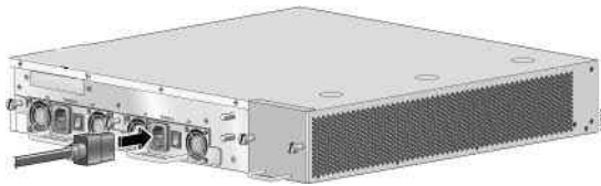
Figure 4-14: Connecting the AC Power
