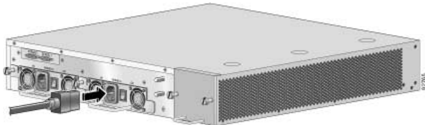
Figure 11: Connecting the AC Power
