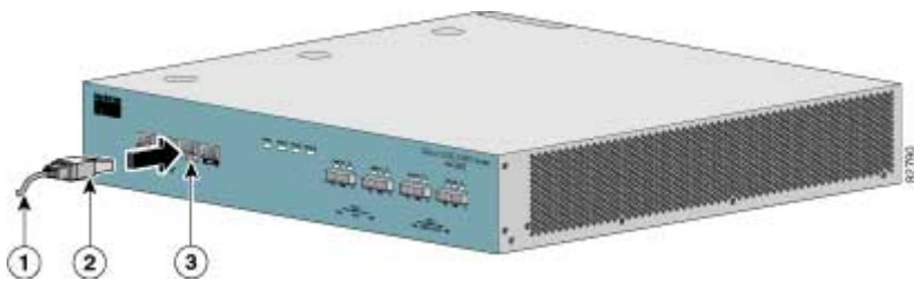
Figure 12: Connecting to the Local Console
