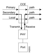
Figure A-3 Secondary Configuration Control Element State
