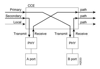
Figure A-5 Thru Configuration Control Element State
