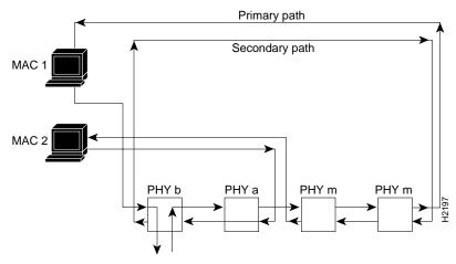
Figure A-10 Wrap-S Configuration State
