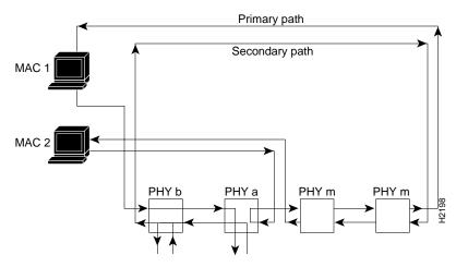
Figure A-11 Wrap-A Configuration State
