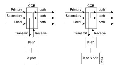
Figure A-6 Concatenated Configuration Control Element State
