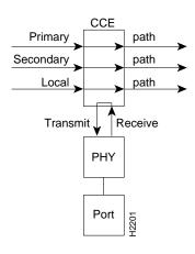
Figure A-4 Isolated Configuration Control Element State
