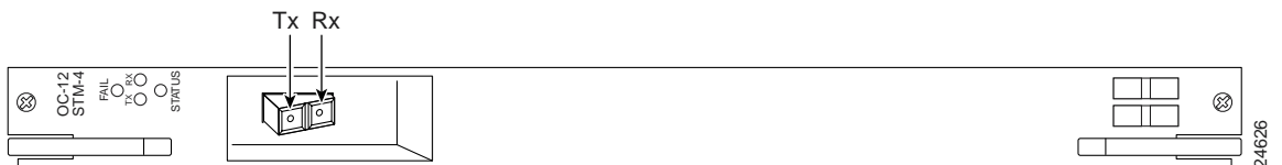
Figure B-8 Cisco 6400 OC-12 NLC Card
