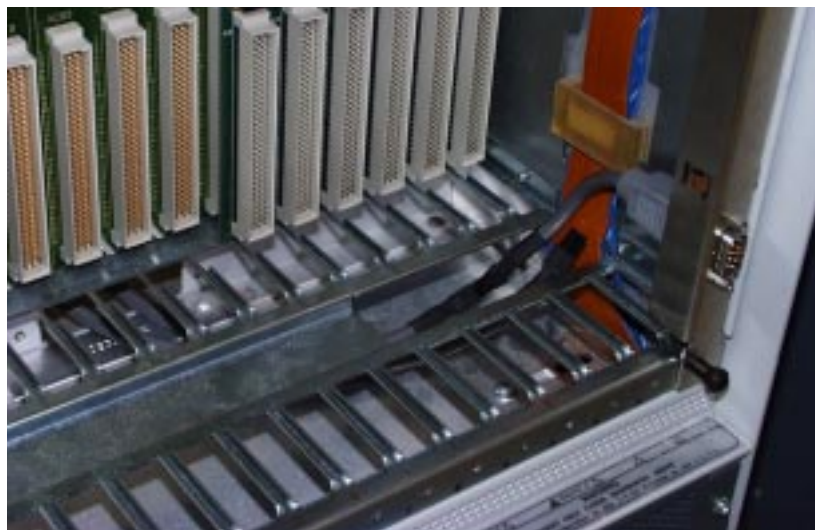
Figure 7 Rear Chassis Cable Routing (VCO/20 and VCO/4K with Serial Number less than MHT03400016)
