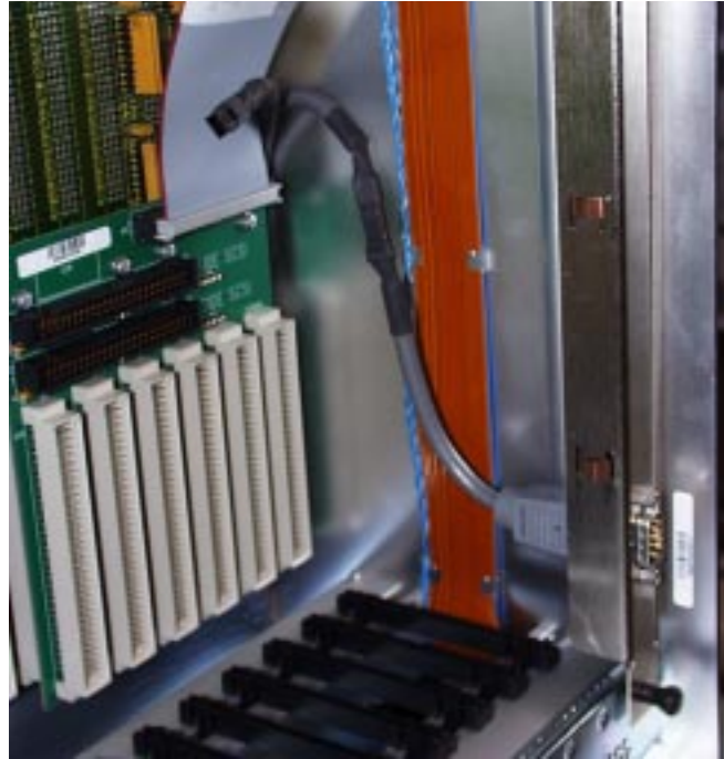
Figure 6 Rear Chassis Cable Routing (VCO/4K with Serial Number MHT03400016 and Higher)
