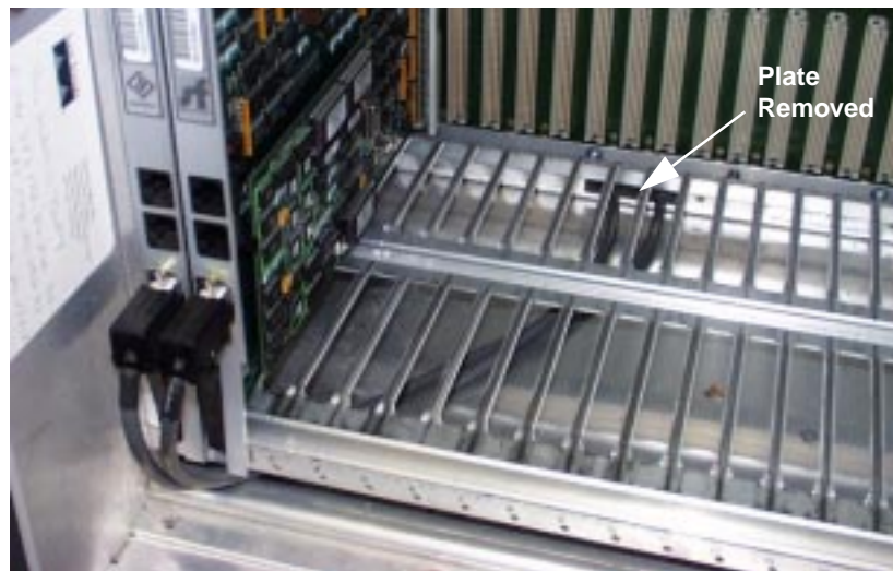
Figure 5 Long Cable Section Installation (VCO/20 and VCO/4K with Serial Number less than MHT03400016)
