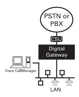
**Note:** A CSU is required if you are connecting to the PSTN or if the Gateway is more than 30 meters from a PBX.
