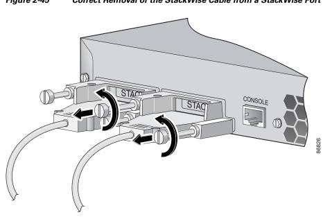
Figure 2-45 Correct Removal of the StackWise Cable from a StackWise Port
