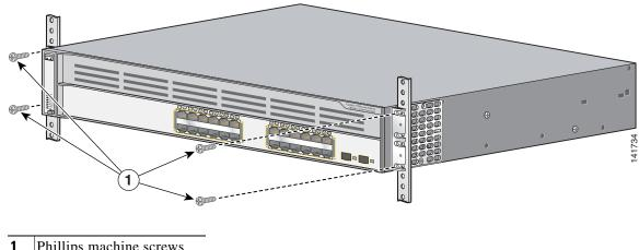
Figure 2-37 Mounting the Catalyst 3750G-24WS-S25 and 3750G-24WS-S50 Switches in a Rack
