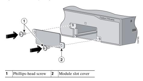
Figure 2-54 Replacing the XENPAK Module Slot Cover
