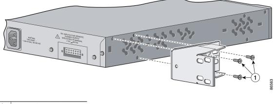
Figure 2-31 Attaching Brackets for 24-Inch Racks, Rear Panel Forward
