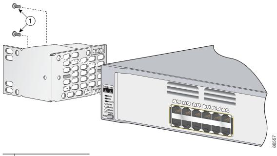
Figure 2-15 Attaching Brackets for 24-Inch Racks, Front Panel Forward
