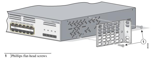
Figure 2-19 Attaching Brackets for 24-Inch Telco Racks
