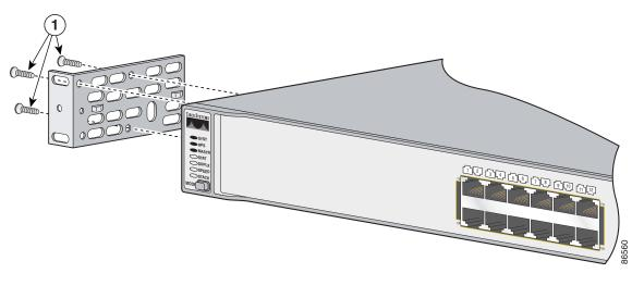
Figure 2-24 Attaching Brackets for 19-Inch Racks, Front Panel Forward
