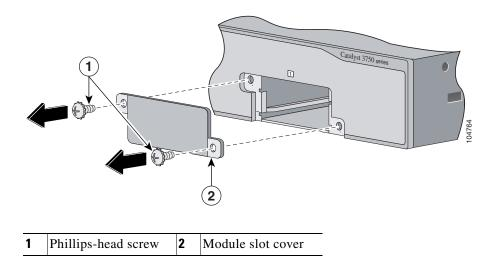
Figure 2-51 Removing the XENPAK Module Slot Cover
