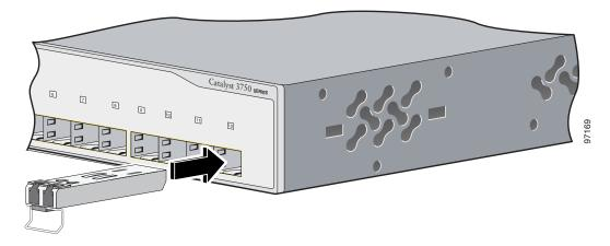
**Step 5** For fiber-optic SFP modules, remove the dust plugs from the optical ports, and store them for later use.
