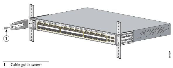
Figure 2-40 Attaching the Cable Guide on the Catalyst 3750 Integrated Wireless LAN Controller Switches
