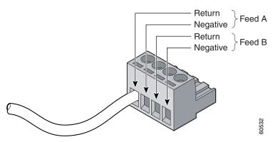
**Step 6** Use a ratcheting torque screwdriver to torque the terminal block captive screw (above the installed wire lead) to 4.5 lbf-in. (72 ozf-in.), as shown in Figure C-8.
