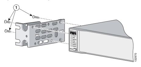
Figure 2-33 Attaching Brackets for ESTI Racks, Front Panel Forward
