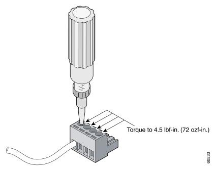
**Step 7** Repeat Steps 4 and 5 for the remaining three DC-input power source wires. Figure C-9 shows the completed wiring of a terminal block plug.
