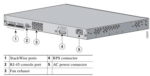
Figure 1-23 Catalyst 3750-24FS Switch Rear Panel
