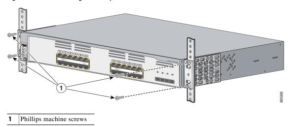
Figure 2-35 Mounting the Catalyst 3750G-24TS Switch in a Rack
