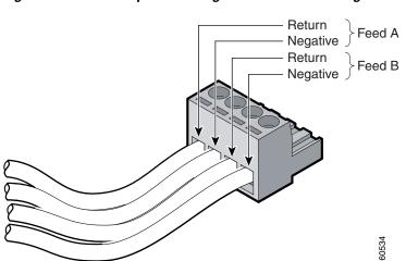
Figure C-9 Completed Wiring of Terminal Block Plug
