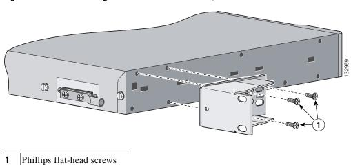
Figure 2-29 Attaching Brackets for 23-Inch Racks, Rear Panel Forward
