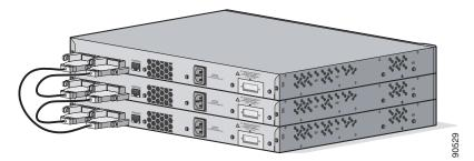
Step 1 Insert one end of the StackWise cable into the StackWise port at the back of a switch. See Figure D-3.
