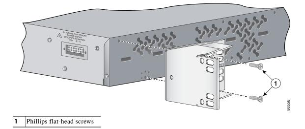
Figure 2-17 Attaching Brackets for 24-Inch Racks, Rear Panel Forward
