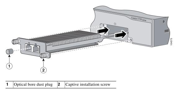
**Step 6** Secure the XENPAK module in place by tightening the two captive installation screws. Do not overtighten the captive screws.
