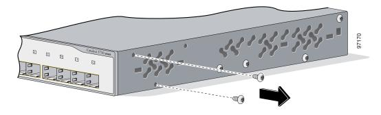
Figure 2-12 Removing Screws from the 3750G-24TS Switch
