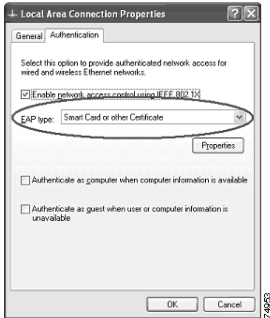
Figure 2-12 Selecting the Authentication Mode in Microsoft Windows XP Professional
