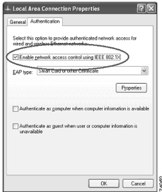
Figure 2-11 Enabling 802.1x in Microsoft Windows XP Professional
